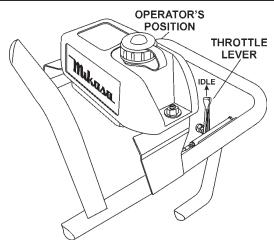
Figure 9. Throttle Lever (Idle)
